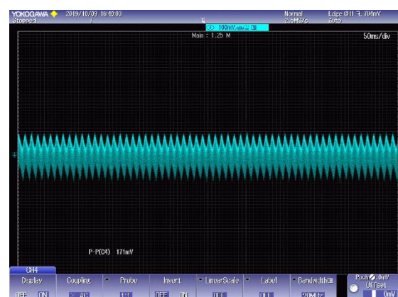
(b) 230 V (measured value=171 mV)
